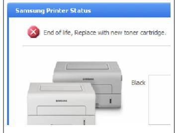
Note: for subsequent refills, it's possible you'll get the "End of life ...." message before fade out. Easy to confirm, because the machine also refuses to print
